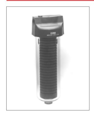
Cuno housings Model 1M1 and 1M2 are constructed from high impact plastic for durability and long service life. The housing's two piece design allows for easy installation and cartridge change-out. The housing is available for one-high (9 3/4") cartridges (1M1) and two-high (19 ½") cartridges (1M2) with transparent or opaque sumps. Both models have maximum pressure /temperature ratings up to 125 psig at 100°F with flow rates to 16 gpm.
