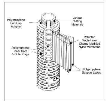
The Electropor II cartridge is extremely durable, and features all polypropylene molded components that Teflon® is a registered trademark of DuPont Incorporated. withstand arduous operating conditions.
