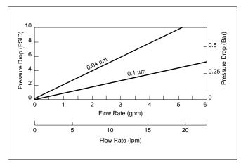
Notes: Flow Rate/Pressure Drop is for a 10" element in 25°C water.
