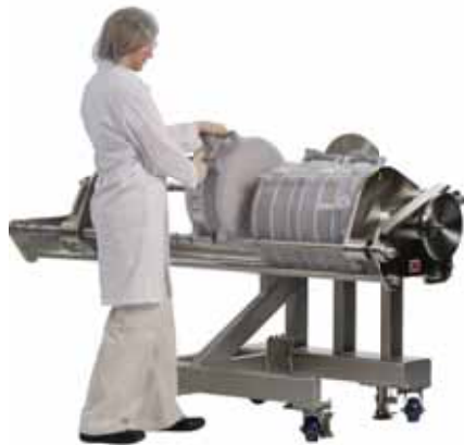
Figure 1. Zeta Plus™ Encapsulated Large Holder Loading Process
